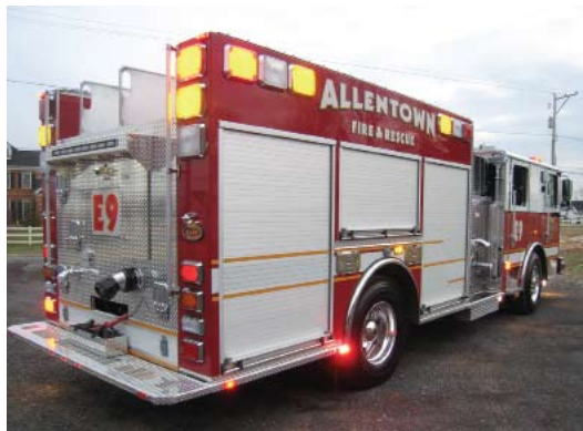
Above: Engine 13 is a KME Severe Service engine with standard lower compartments and an extra can compartment.
